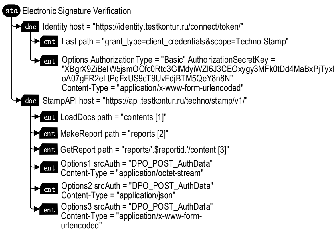
Figure 2 – Specifying cryptographic service entry points as virtual multi-documents in the SODB model
