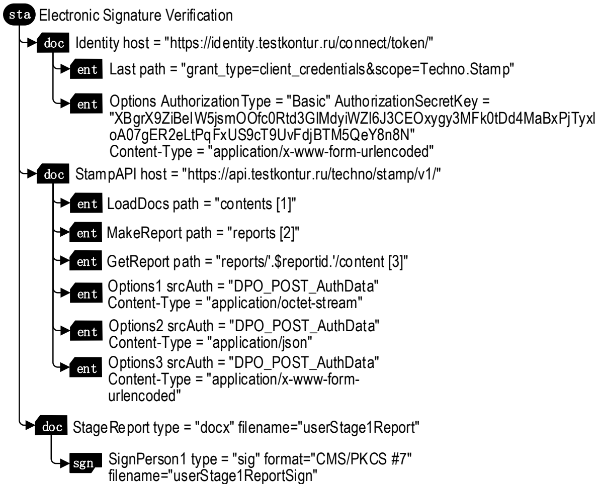
Figure 3 – Fragment of a model with a multi-document that structures the report and its signature with the newly introduced sgn-element
